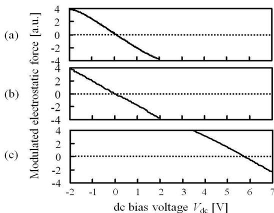
Fig. 1. Modulated electrostatic forces as a function of dc bias voltage between a W-coated cantilever and a Ge(001) surface measured in (a) FM-, (b) heterodyne AM-, and (c) AM-KPFMs. The stray capacitance due to the cantilever strongly influences the surface potential measurements in AM-KPFM, whereas the effect of the stray capacitance on the surface potential measurements is almost removed in heterodyne AM-KPFM.
