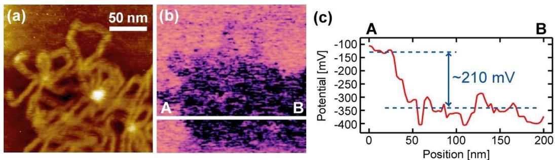
Figure 1. (a) Topographic and (b) potential images of DNA adsorbed on mica taken in 1 mM HEPES/0.1 mM  $\text{NiCl}_2$ . (c) Potential profile measured along Line A-B in (b).
