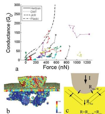
(1) Tunneling to contact  $I(z)$  of W tip with Au(111) surface at 150K; (b) local tip changes (red/green colour for adsorbed/evaporated atoms) due to contact with Au(111) near the center of the FIM image.
