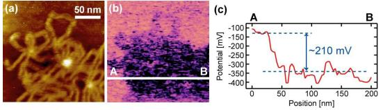
Figure 1. (a) Topographic and (b) potential images of DNA adsorbed on mica taken in 1 mM HEPES/0.1 mM NiCl<sub>2</sub>. (c) Potential profile measured along Line A-B in (b).
