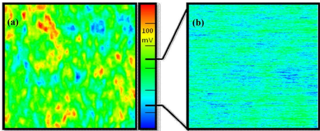
**Figure 1:** KPFM potential map of (a) SiO<sub>2</sub> surface and (b) BN surface. Images are 1  $\mu\text{m}$  x 1  $\mu\text{m}$  in size.
